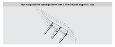
Carry out the assembly for the pushing points by following the installation sequence in Section 5.1
